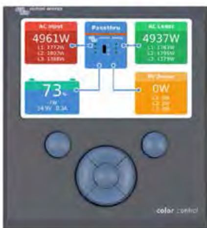
Color Control Panel, showing a PV application
